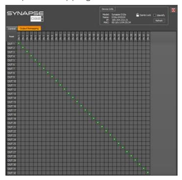
The D32o can have the Dante™ input channels remapped to customized analog outputs on the device. Changes are made by simply clicking the desired input/output selection on the grid. The green indicator will show the connection has been made. By default, the input channels are paired to their corresponding outputs of the same values.
