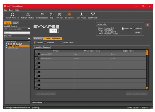
In standard mode, up to 32 Dante<sup>™</sup> audio channels can be assigned to the DM1 receivers using Dante<sup>™</sup> Controller. The user can then select which one of the assigned channels to listen to by navigating through and selecting the desired one from the front panel controls once they have been assigned.
