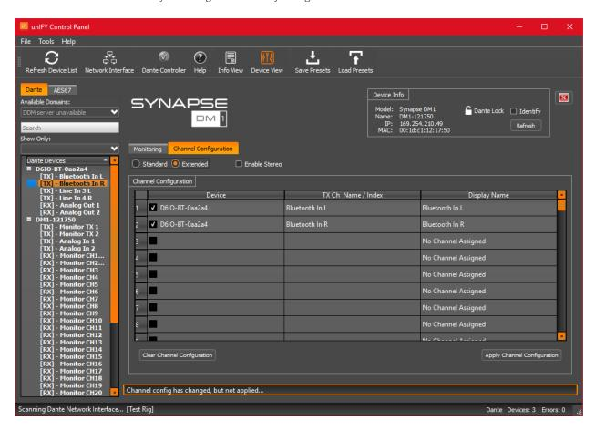
In extended mode, instead of the user selecting from channels already routed over the network to the DM1, the DM1 can use dynamic audio routing of networked audio instead. When a user selects an available channel using the front panel controls, the device will dynamically set up a route for that audio.
