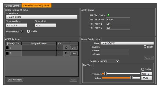
The stream control tab shows the various settings to configure both transmit streams for the unA6IO and receive steams to the unA6IO. There are also some device settings such as device name and IP address configuration.
