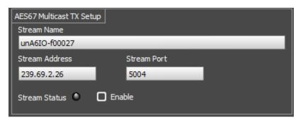
The parameters in this section are used to define the transmit stream from this device. By default, the audio transmitter is turned off. The stream comprises of five channels. The first four channels are the audio from the local analog inputs in order and the fifth is a diagnostic pilot tone.
