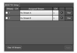
The AES67 Rx setup section allows the user to see and/or select which stream and specifically which channel within a stream is allocated to each analog output. For each output, the current settings for assigned stream and channel are shown, as well as an indication if the assigned stream is active and also if that output is muted or not (the mute control is a duplicate of the output mute control on the Device Control tab).
