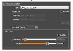
The device configuration shows the various device wide settings. This includes the devices name and IP address, and the settings for the pilot tone.
