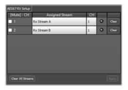
The AES67 Rx setup section allows the user to see and/or select which stream and specifically which channel within a stream is allocated to each analog output. For each output, the current settings for assigned stream and channel are shown, as well as an indication if the assigned stream is active and also if that output is muted or not (the mute control is a duplicate of the output mute control on the Device Control tab).
