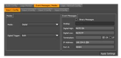
As an example, the event message configured in the example above would result in an event message to be sent to UDP or TCP/IP port 49494 of IP address 169.254.0.200 every time Input 1 changes its digital state. If the state changes from low to high, a "MUTE ON<CR>" message is sent. If the state changes from high to low, a MUTE OFF<CR> message is sent.
