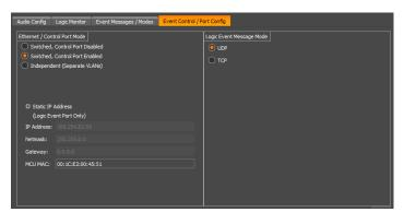
The Logic Event messaging and physical Ethernet ports can be configured to support various AV and control network architectures.
