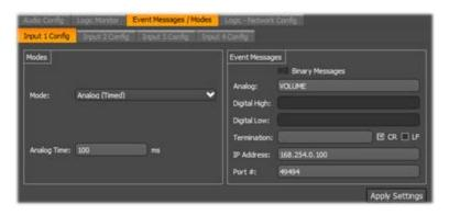
As an example, the event message configured above would result in a UDP event message being sent to port 49494 of IP address 169.254.0.100 every tenth of a second where the data payload of the message would range from VOLUME 0<CR> to 4095<CR> depending on the current input level.
