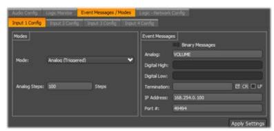
For example, take the message setup as configured in the example above. The "Analog Steps" setting is at 100 so each step size equate to 4096 / 100 = 40.96. This is rounded up to 41. If the volume starts out at a value of 150, that is in step 3 as it's between the values 123 (41 \* 3) and 164 (41 \* 4). While the voltage remains in that range, nothing happens. However, if the value were to
