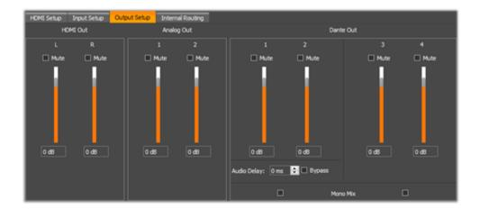
Each channel features independent volume control and mute functions with a mono mixdown option for the Dante<sup>TM</sup> output channels.
