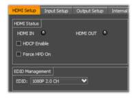
The unHX2D allows HDMI audio sources to be de-embedded and reembedded from/to the HDMI I/O on the device. The HDMI Setup controls all the following configuration and status monitoring.
